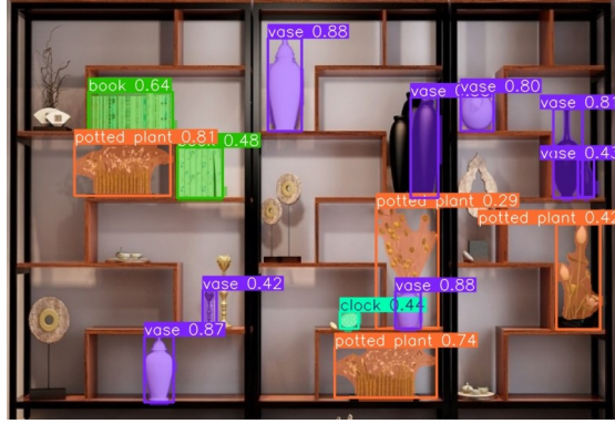
Fig. 2. Example for object recognition of YOLOv8
